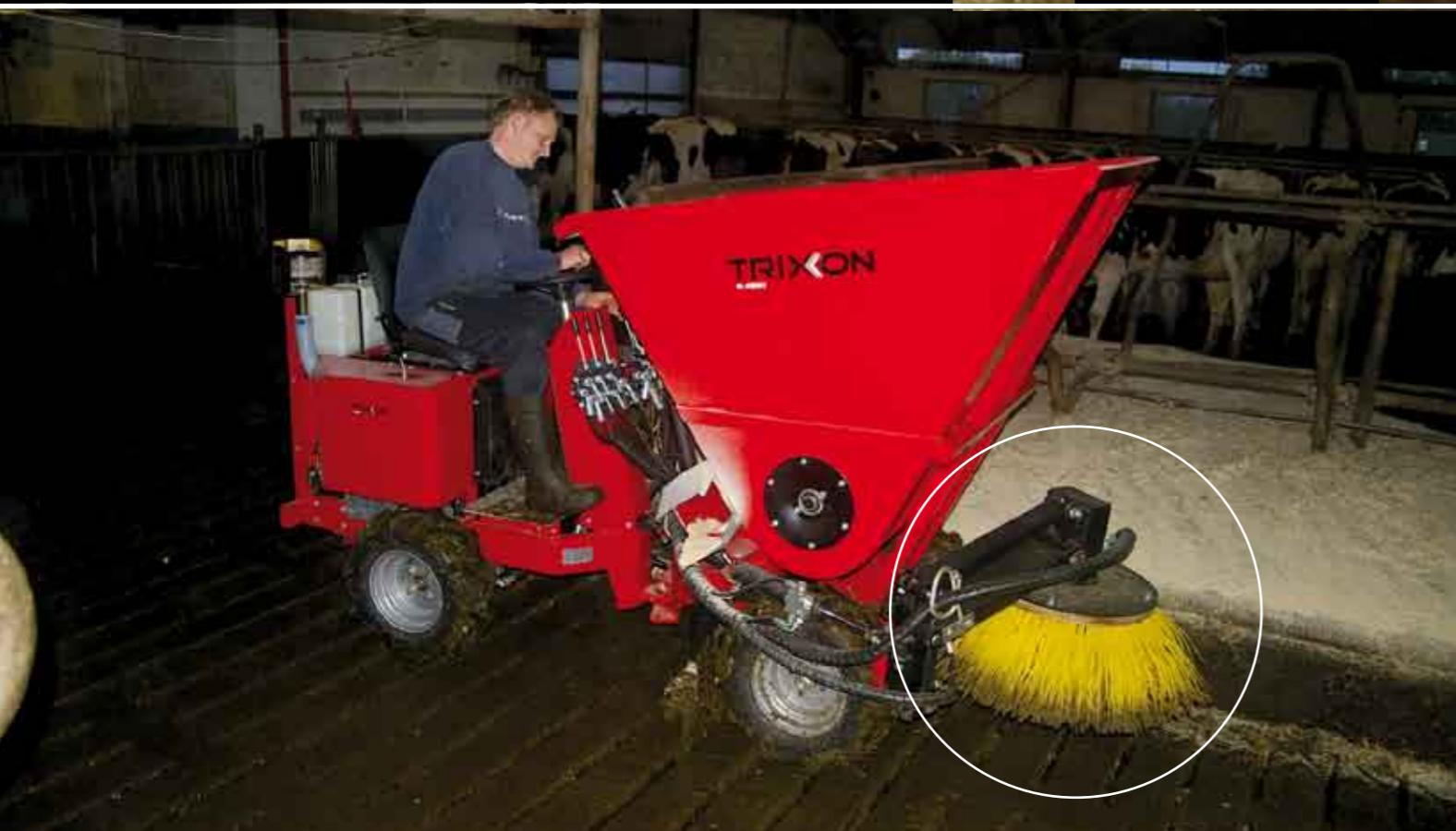
The broom diameter is 800 mm (31 inches) and is hydraulic adjusted both up and down and to the sides. This ensures effective cleaning in all corners.
